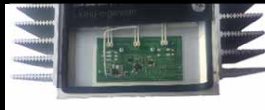
SES Lighting radio dimming transmitter
